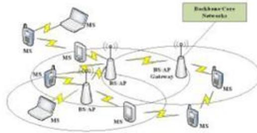
Fig [3]: Mesh Architecture Networks
