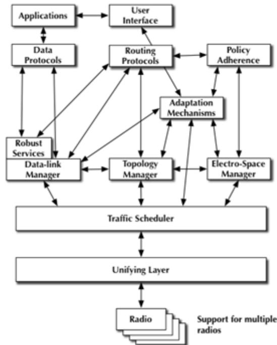
Fig [5]: Cognitive Radio Software Architecture [6]
