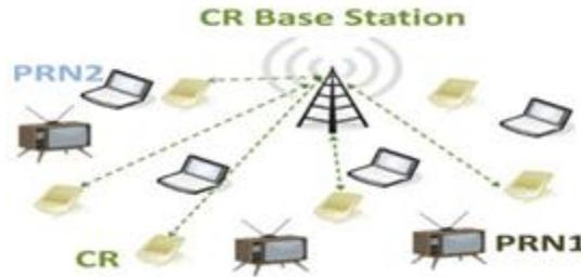
Fig [2]: centralized infrastructure based-CRN
